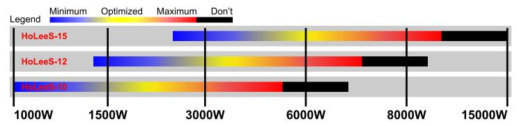
**Blue** (**Minimum**): If you are powering your sub in this range, it will operate comfortably with zero strain or fatigue. Power ranges this low will not damage your speaker, but it wont capture the Subzero full capabilities.
