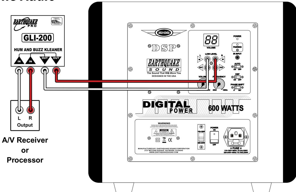
**Connect the GLI-200 between the A/V Receiver/Processor and a powered subwoofer via RCA cables.**
