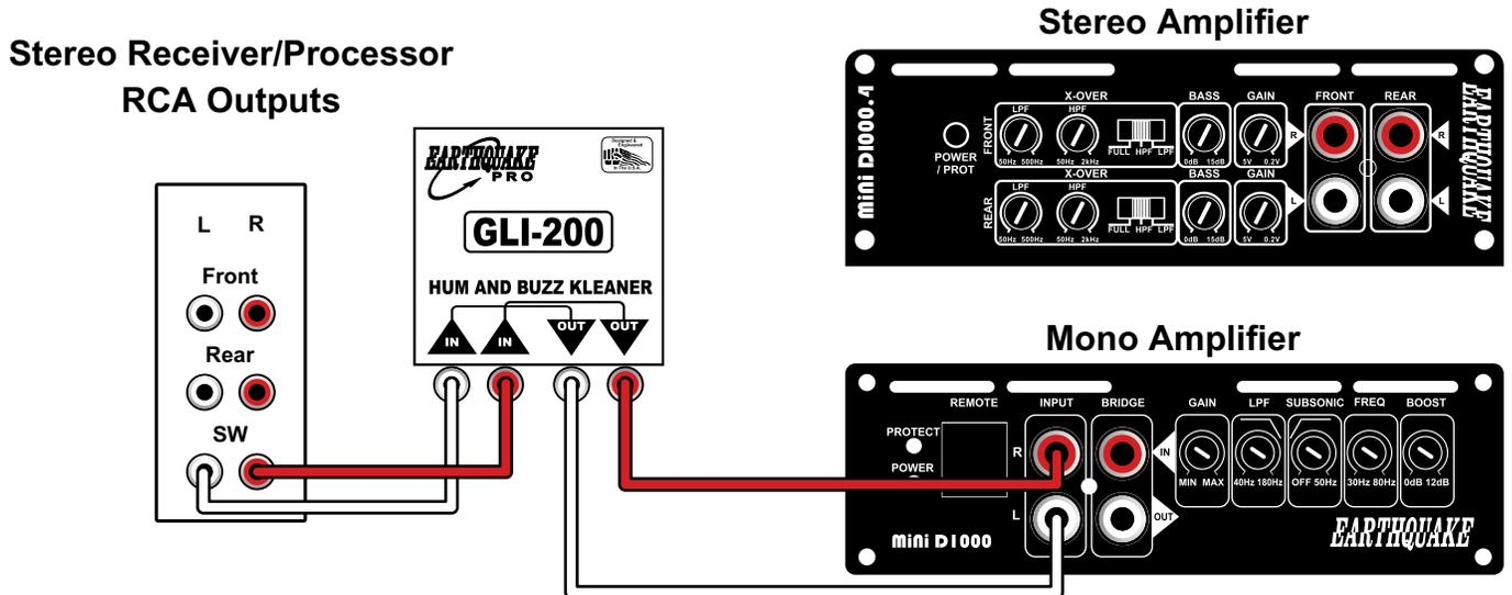
Connect the GLI-200 between the stereo receiver/processor front, rear, or sub outputs and a stereo or mono amplifier inputs via RCA cables.
