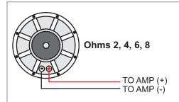
If using SINGLE 2 OHM coils the total load would be 2.0 ohm If using SINGLE 4 OHM coils the total load would be 4.0 ohm If using SINGLE 6 OHM coils the total load would be 6.0 ohm If using SINGLE 8 OHM coils the total load would be 8.0 ohm
