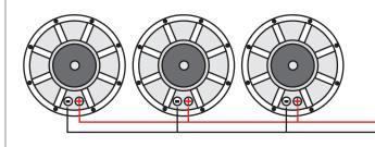
If using SINGLE 2 OHM coils the total load would be .66 ohm If using SINGLE 4 OHM coils the total load would be 1.3 ohm If using SINGLE 6 OHM coils the total load would be 2 ohm If using SINGLE 8 OHM coils the total load would be 2.7 ohm
