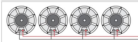
If using SINGLE 2 OHM coils the total load would be 0.5 ohm If using SINGLE 4 OHM coils the total load would be 1.0 ohm If using SINGLE 6 OHM coils the total load would be 1.5 ohm If using SINGLE 8 OHM coils the total load would be 2 ohm
