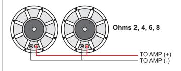
If using SINGLE 2 OHM coils the total load would be 1.0 ohm If using SINGLE 4 OHM coils the total load would be 2.0 ohm If using SINGLE 6 OHM coils the total load would be 3.0 ohm If using SINGLE 8 OHM coils the total load would be 4.0 ohm
