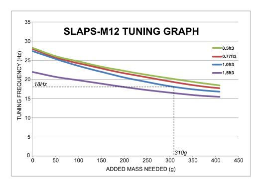
If you decide to modify the mass provided, every 1/2" drill hole (±9g) will increase the tuning frequency by 1Hz. Additionally, keep the modifications in symmetry to allow even mass distribution.
