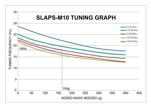
For example, the net internal volume of your speaker box is 1 cu.ft. (28.3L) and your preferred tuning frequency is 18Hz. Then you will need to add about 164g of mass to the SLAP-M10 or add about 310g of mass to the SLAPS-M12.
