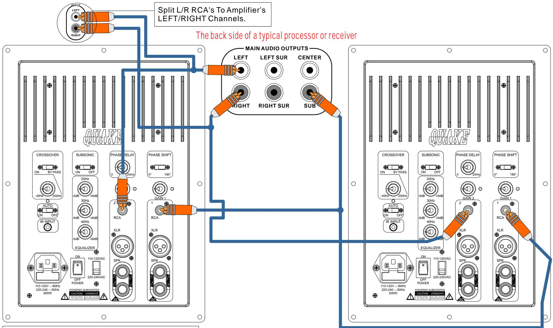
The same wiring configuration can be duplicated for the XLR inputs. NOTE: We provide three different input types, but do not recommend mixing input types.
